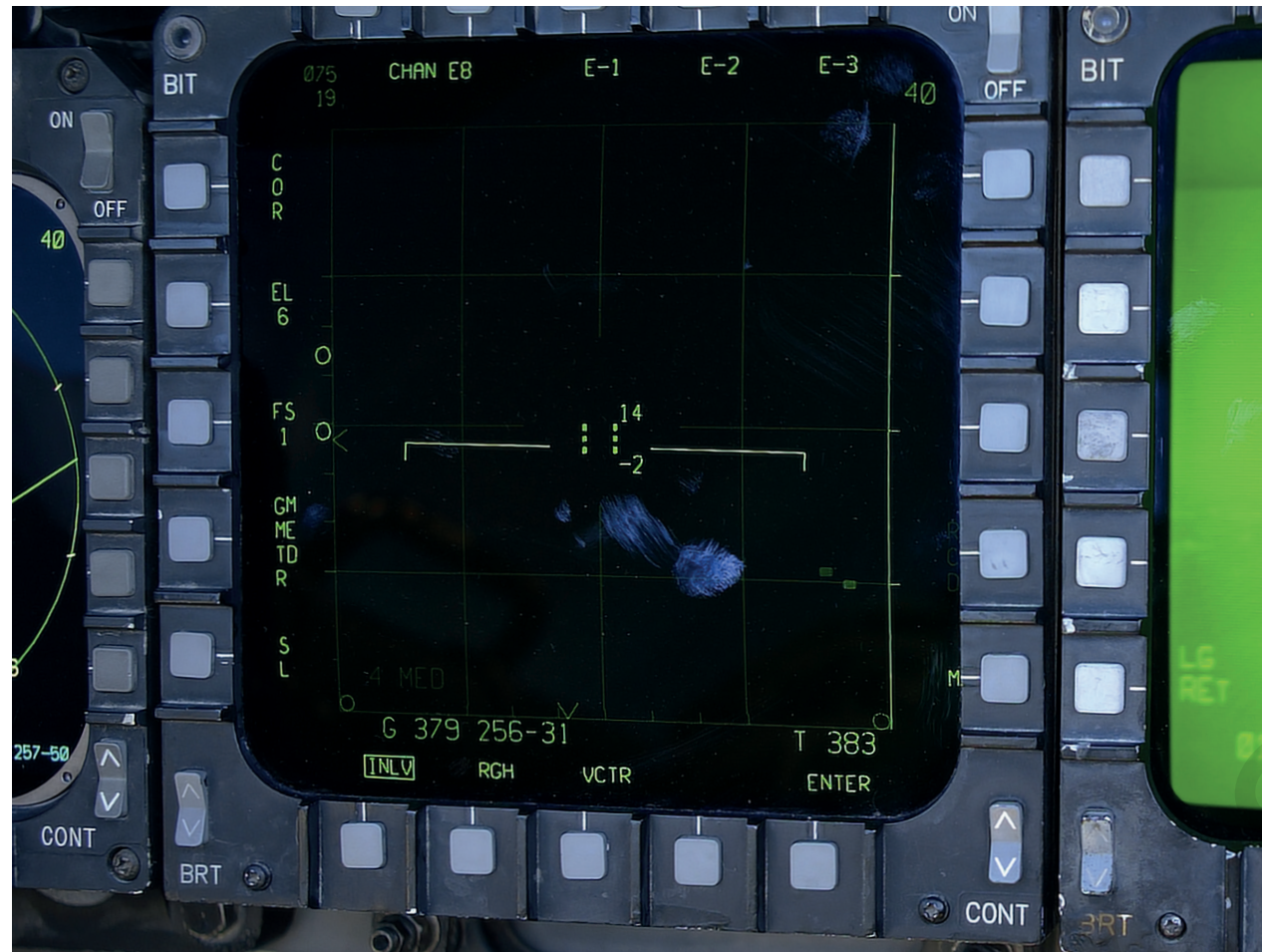
ABOVE The APG-70, Suite 4E+, in search mode. Note the COR and SL options at PB1 and PB5, respectively. (Author)
